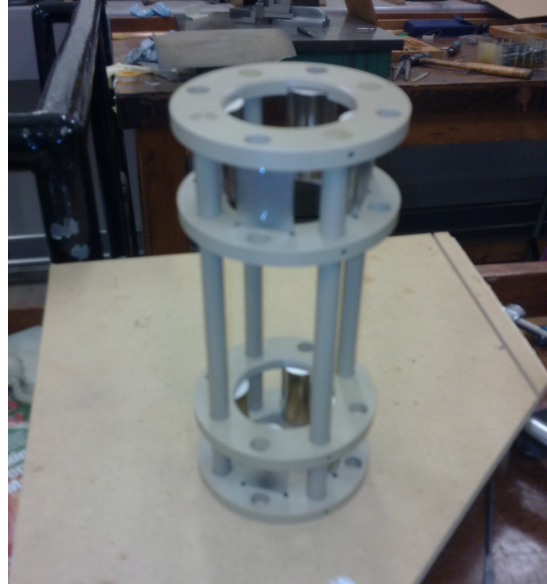
Figure 5.9: Quadrupole doublet - the Quadrupole doublet designed according to the specification from the simulations. The electrodes are the small metal half cylinders at the top and bottom, the rest is the PEEK support structure
